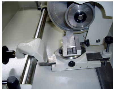
Spanbrechernuten- Schleifapparat chip breaking groove grinder
